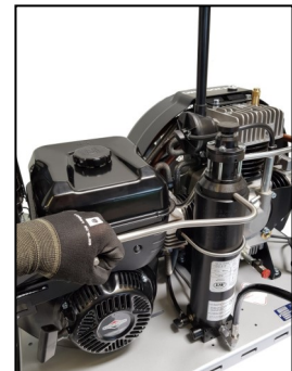
Fig. 1 Loosen Filter Housing Cover by using the Filter Key
