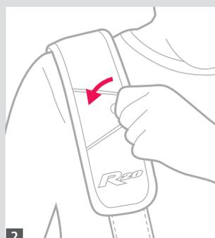
**2** Open the flap on the right shoulder strap to access the release cord.
