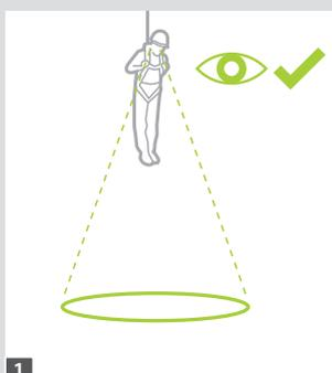
**1** Check the ground below to ensure descent path is clear and a safe landing is possible.
