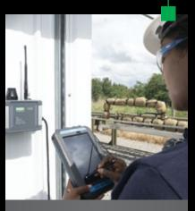
The MSA HUB allows up to 16 ALTAIR io360 Gas Detectors to form a network you manage locally via the Safety io Grid mobile app.
