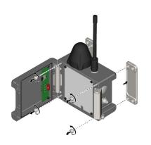
(7) Remove the four screws and the wall brackets at the back of the housing.
