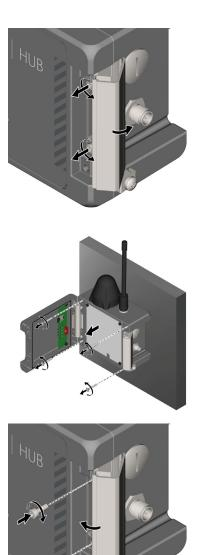
(4) Open housing by opening the right joints and unscrew the lid screws using a Torx T20.
