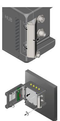
(5) Open housing by opening the right joints and unscrew the lid screws using a Torx T20.
