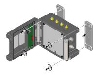
(8) Remove the four screws and the wall brackets at the back of the housing.
