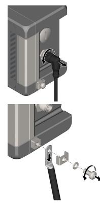
(1) Unplug the power plug and remove Ethernet cable, if present.
