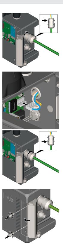
(6) Tighten upper nut with a torque of 7.5 Nm. The cable gland is fixed in the housing.
