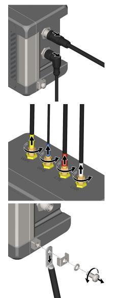
(1) Unplug the power plug and remove Ethernet cable, if present.
