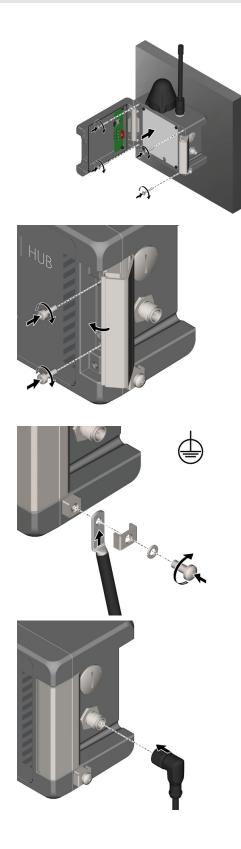
**Note:** If no wall brackets are used, mount the device to the surface directly. Use four appropriate screws and apply a torque of 5 Nm.
