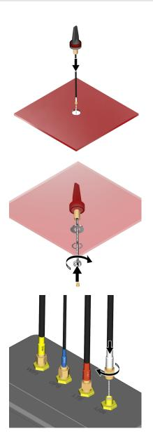
(13) Pass the antenna cables through the hole. **Note:** Metal-to-metal contact between the mounting surface and the mount is essential for best performance of the antenna.
